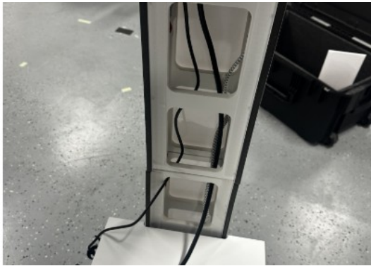
Cable channels in kiosk leg — cables routed through
